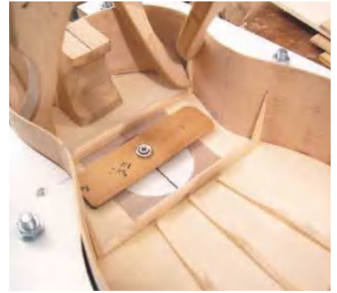
STEP 20. Clamping the long tentellones
